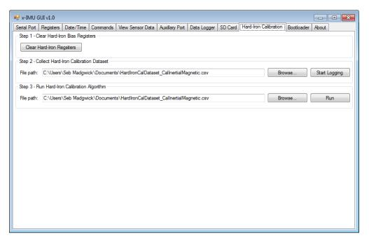
Figure 22: x-IMU GUI hard-iron calibration tab page
