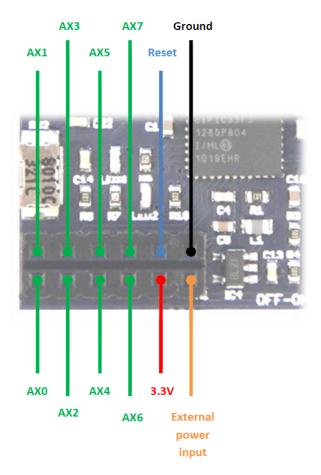
Figure 23: Auxiliary port pins
