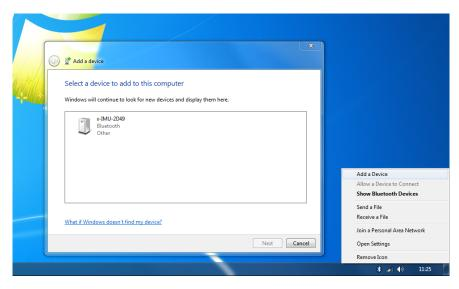
Figure 19: Searching for the x-IMU as a new Bluetooth device in Windows 7
