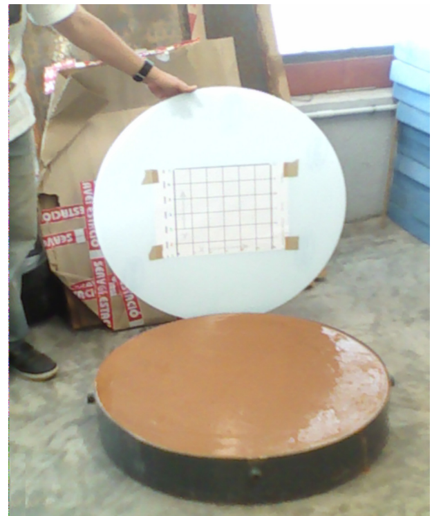
FIG. 3 Specimen and PMMA plate with grid to guide the device.
