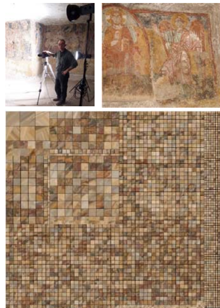
Figura 5.21: UV automáticas. Fuente: BERALDIN, J-A, Virtualizing a Byzantine Crypt by Combining High-resolution Textures with Laser Scanner 3D Data, VSMM 2002 Schedule, Date: 25~27 September 2002, Venue: Hilton Hotel, Gyeongju, Korea
