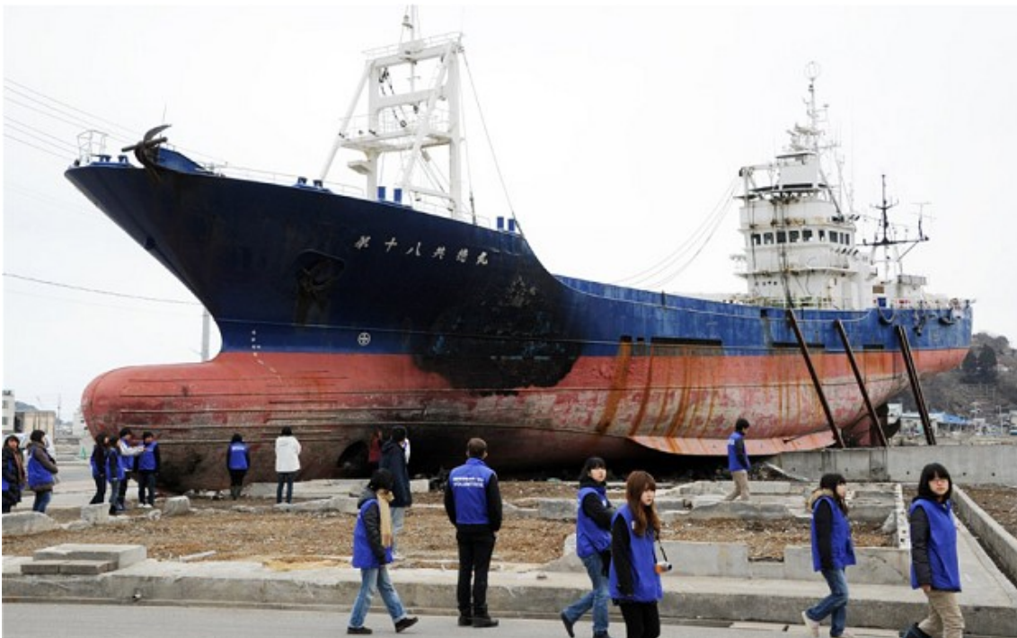
Figure 21: Photo of the 330-tonne Kyotokumaru, a fishing boat 60 m long that was swept 750 m inland when the tsunami reached the shoreline in Kesenuma (Japan, 2011). It may be observed that the structure of the ship has not suffered major damage (photo www.telegraph.co.uk ). However, it was scraped.
