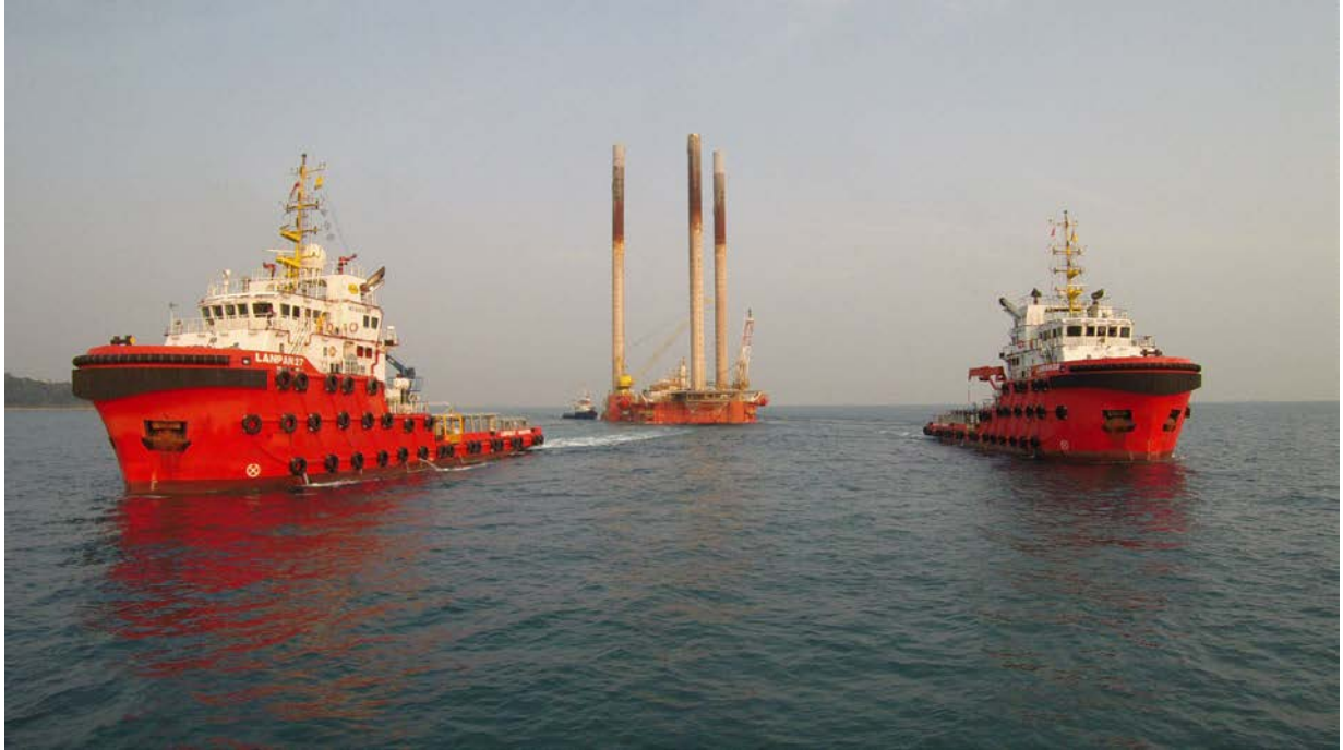
Figure 26: Oil Platform CENDOR MOPU being towed this time successfully in 2014 from Malaysia to Batam, Indonesia (photograph from http://www.marinelink.com/news/successful-completion381631.aspx ). The legs standing some 90 m over the water may be observed. It seems that the stability of the legs could have been enhanced by staying diagonal cables between them (making the system more rigid, which do not seem to exist in the photo).
