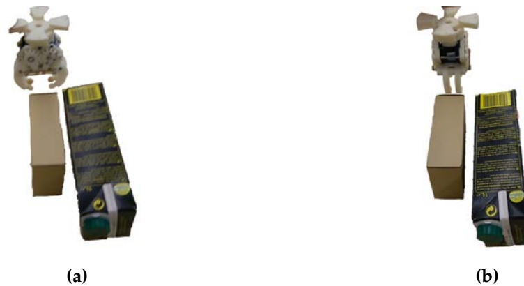
Figure 4.12: Possible pushing poses for push an object along its principal axis - In Figure 4.12a the closing direction of the gripper is orthogonal to the pushing direction, and for the case depicted in the figure the gripper will likely push also the black juice box. In Figure 4.12b the closing direction of the gripper is parallel to the pushing direction.
