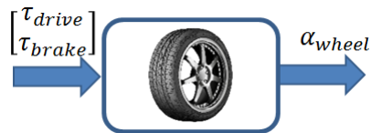
Figure 3.7: Wheel dynamic model diagram
