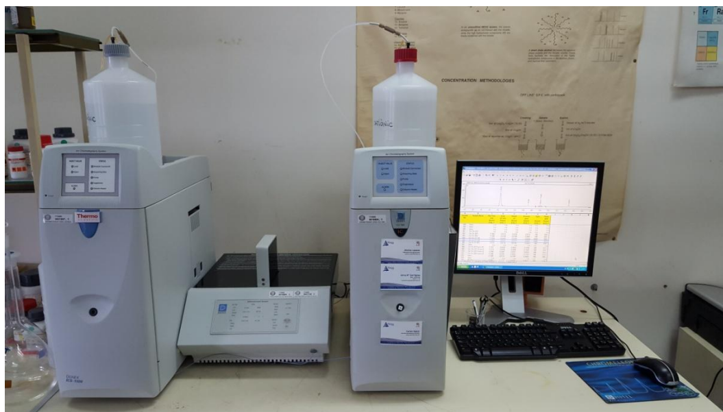
Figure 5-2. Dionex ICS-1000 Ionic Chromatography System
