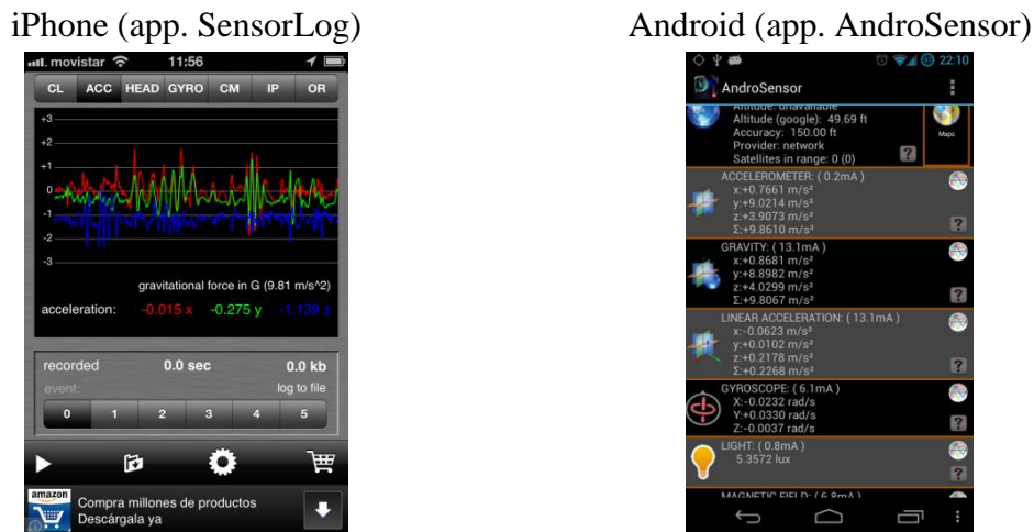
Fig. 2 – Smartphone's raw accelerometer and gyroscope measurements in different platforms
