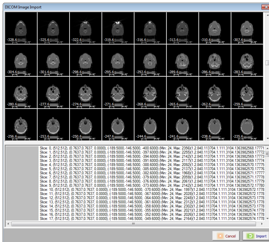
Figure 4.10: DICOM Image Import dialog. The gray scale is mapped into each image Hounsfield number range.
