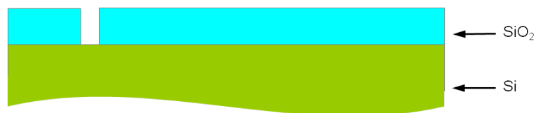
Figure 5.31: Second resin lift-off.
