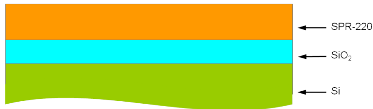
Figure 5.28: Resin SPR-220 1.2, thickness 1 \mu\text{m} .
