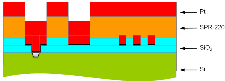
Figure 5.43: Platinum sputtering for PADs, thickness 100 nm.
