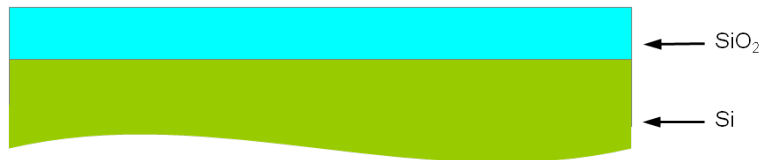
Figure 5.26: Silicon oxide, thickness 120 nm.
