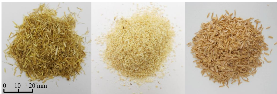
Figure 5.1. Barley straw fibres, corn pith aggregate and rice husks used as raw materials.
