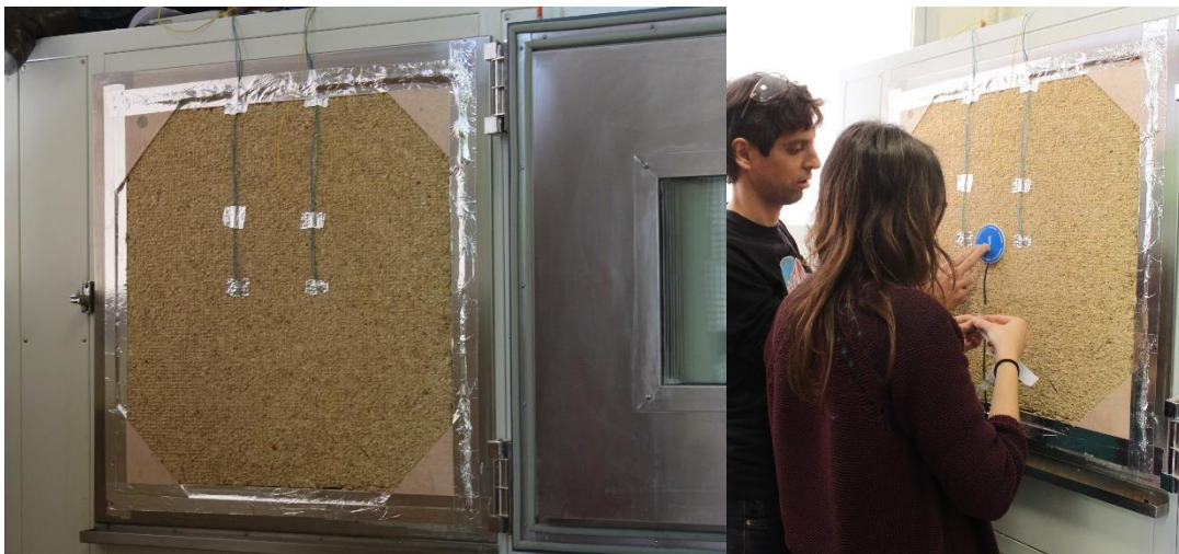
Figure 4.3. Experimental set-up used for the specimens of different ETIC systems. The specimens were fixed at the opening of the climate chambre (left) and covered with an isolated box (right).
