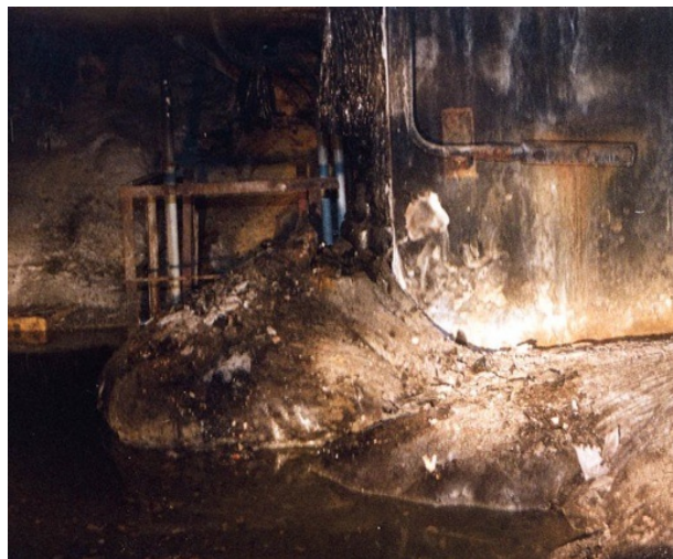
Figure 6.2: A blob of corium in the Chernobyl Nuclear Reactor. From [1].
