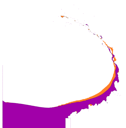
Figure 3.69: Collapse of a water column over a rigid step. Superposition of the 2D results obtained at t = 0.3s with the mesh with average size 0.002m for the slip (orange colour) and the stick (pink) conditions.
