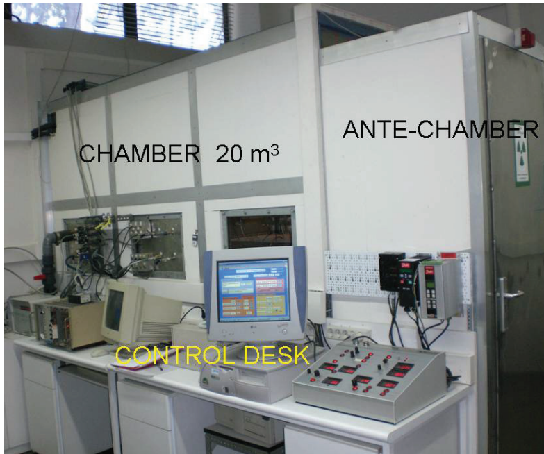
Figure 3.1: The radon chamber at the INTE laboratory (UPC) is presented here with its control panel
