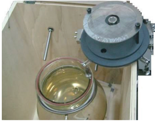
Figure 2.7: Detection volume of the electrostatic sphere ARMON used for ^{222}\text{Rn} concentration measurements in the atmosphere. The spherical detection volume is illustrated together with the volume cap which is made up of a wire screen with a PIPS detector located at its center
