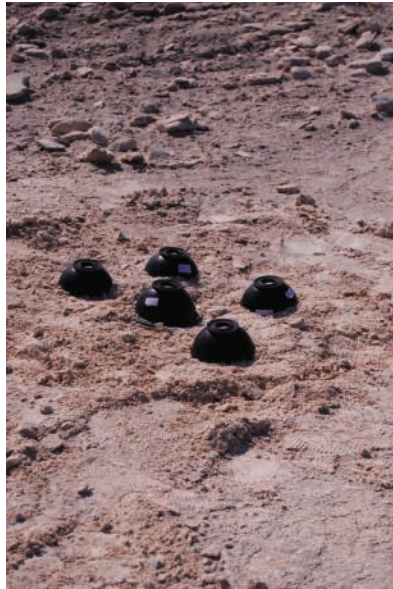
Figure 6.3: Typical measurement of ^{222}\text{Rn} flux by EIC E-Perm monitors at the unrestored area (Zone 3) at the Huelva phosphogypsum pile.
