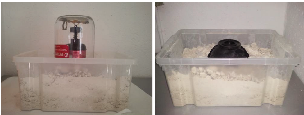
Figure 4.1: Reference method for radon flux study on the exhalation bed (on the left) and RT-EIC radon flux monitor measurement (on the right).
