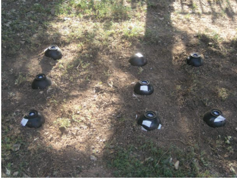
Figure 2.5: Classical EIC monitors configuration for radon flux measurement at Los Pedrones site (Spain).
