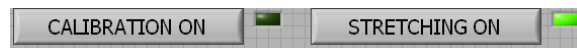
Figure B.1: It can be seen from the figure that calibration state is off as the LED is not glowing while stretching state is on because the LED is glowing.
