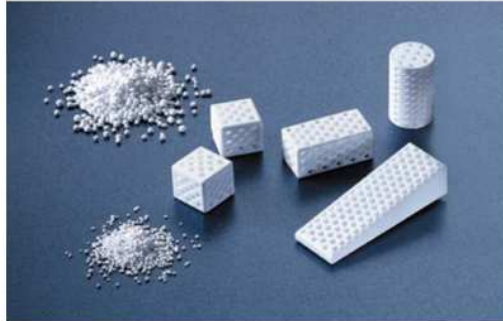
Figure 1.13. Examples of calcium phosphate-based bone substitution materials (from [10]).
