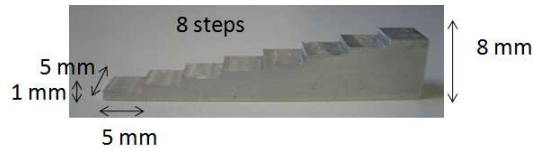
Figure 7.7. Aluminum step-wedge used as a standard of the radiopacity tests. The step-wedge was made at the Mechanical Workshop of the Department of Material Science and Metallurgy of the Technical University of Catalonia.
