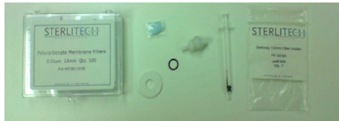
Figure 3.4. Syringe, filter holder and filters (pore size of 0.01\ \mu\text{m} ) used to remove any present colloidal \text{SiO}_2 after soaking the samples.
