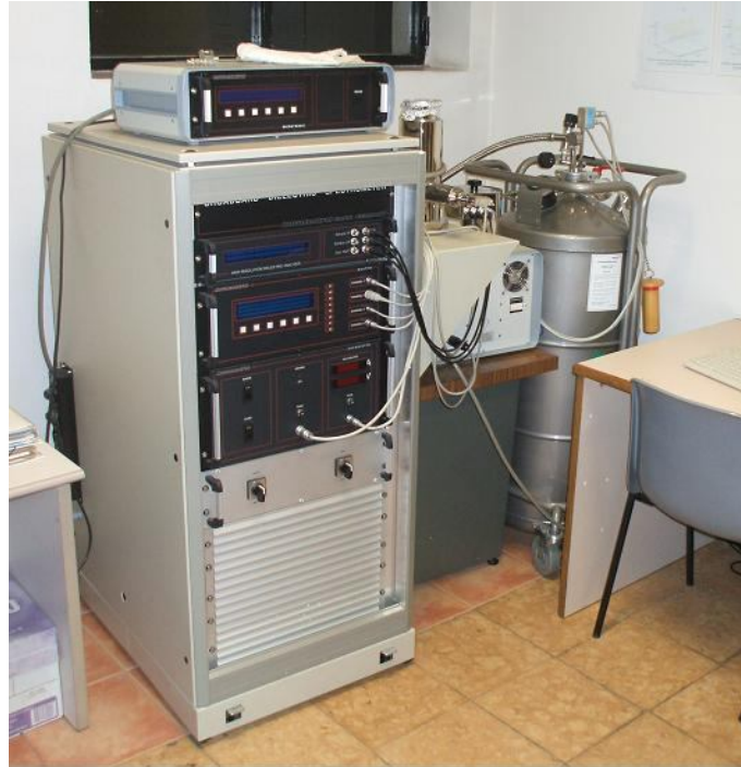
Figure 4.22. BDS40 spectrometer with a Novotherm temperature control system.
