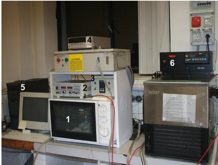
Figure 4.15. A TSDC experimental setup: (1) DeLonghi forced air oven; (2) Heizinger LNC 30000-2 high voltage source (0–30kV); (3) Eurotherm 808 PID temperature programmer; (4) Keithley 6514 electrometer; (5) computer with an analog-to-digital port; (6) Huber CC-245 refrigeration bath.
