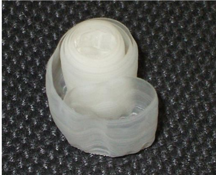
Figure 4.23. XLPE ribbon obtained from a MV cable using a lathe
