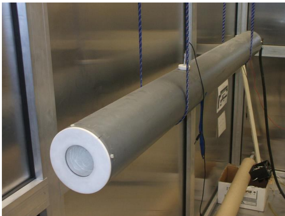
Figure 4.29. Oven used to anneal and to polarize long samples at high temperatures prior to PEA space charge measurements.
