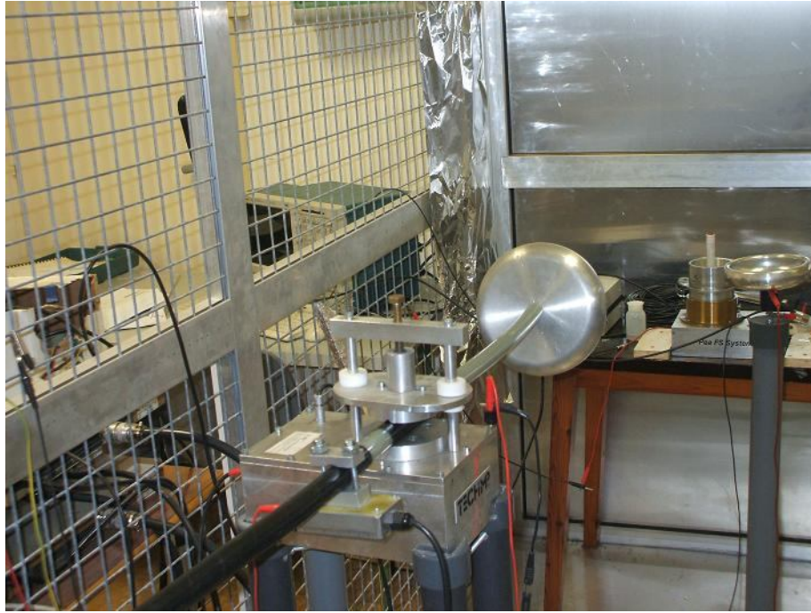
Figure 4.26. Techimp PEA Cable measurement system.
