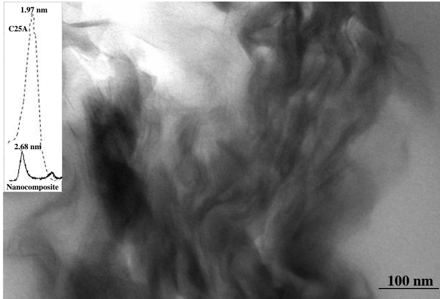
Figure 5.5.1 Transmission electron micrograph showing the morphology of the poly(glc- alt -amh)/C25A nanocomposite with a Cloisite concentration of 3%. Inset shows the diffraction peak associated to the interlayer spacing observed in the C25A organo-modified clay (dashed line) and the nanocomposite sample (solid line).
