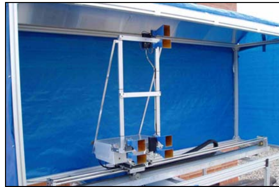
Fig. 4.25: Photo of the gbSAR UPC sensor located on the roof of the TSC department at the UPC.
