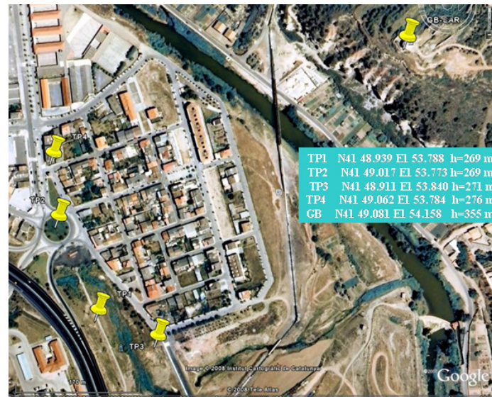
Fig. 5.14: Location of the four tie-points used for the estimation of UPC gbSAR's trajectory \xi in the Sallent test-site.
