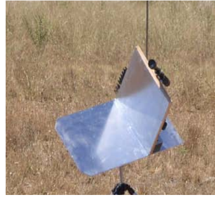
Fig. 4.18: Picture of the Bruderhedral constructed in the laboratory of the UPC ( d_1=65 cm, d_2=55 cm, d_3=45 cm r=2 m). The optical pointer is used to achieve the correct alignment with the sensor location.
