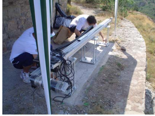
Fig. 4.31: Picture of the concrete basement guaranteeing the observation of the Sallent test-site under a fixed geometry.
