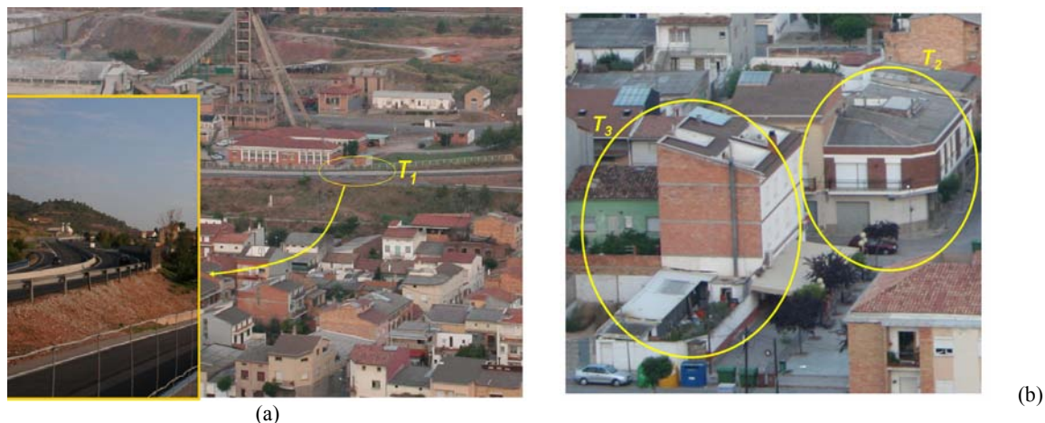
Fig. 7.18: Pictures of the three high reflectivity scatterers selected for the long-time analysis: T_1 (a) is a part of a concrete wall separating the two lanes of the highway close to the urban area; T_2 and T_3 (b) are two close buildings located in the center of the Station district of Sallent.
