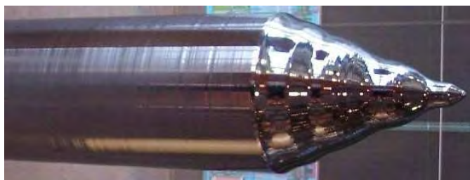
Figure 2.4 Silicon Ingot obtained by Czochralski Crystal Growth Process
