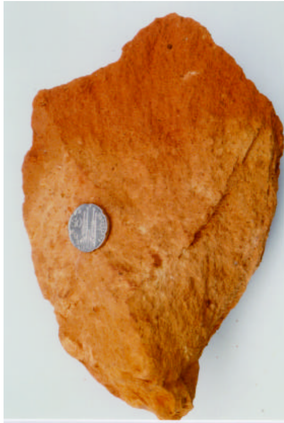
Figure 4.11: Hand sample BI1 representing a baked phonolitic pyroclastic deposit. BI1t has been taken from the upper, reddish part of the sample with a maximum thermal alteration. BI1b has been taken from the lower part with minor effects of thermal alteration.
