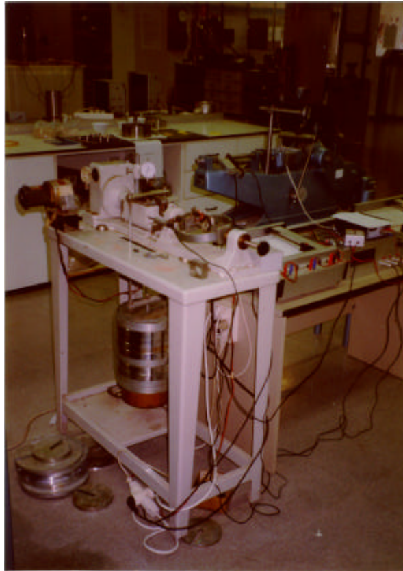
Figure 4.13: Photograph of the small shear test apparatus SHEAR1 used during the geotechnical study.
