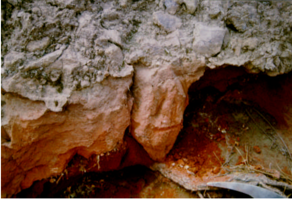
Figure 4.3: Outcrop of residual soil sample RS1. The reddish soil layer is covered and baked by a thick lava flow.
