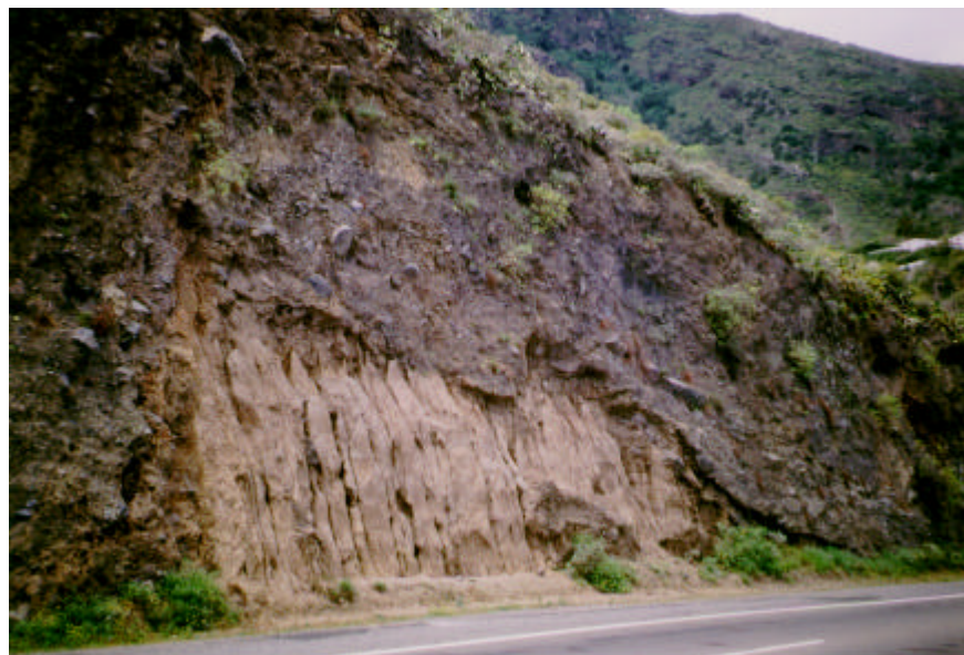
Figure 4.6: Location of the samples of the valley filling breccia EL1 and EL2. The deposit has been generated by a postslide small scale landslide event. EL1 has been taken from the large block of a phonolitic pyroclastic deposit situated in the middle of the deposit. EL2 has been sampled from the matrix of the deposit.
