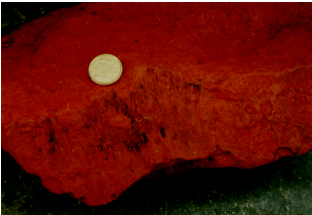
Figure 4.42: Failure zone observed in residual soil RS3. Clear slickenside features are visible characterised by the black colour.
