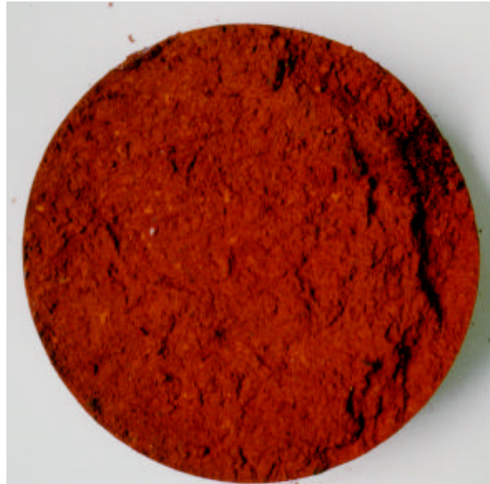
Figure 4.41: Failure zone of undisturbed specimen after a direct shear test applying a vertical stress of 10394 kPa. The failure occurs along a zone characterised by a very irregular morphology. The diameter of the specimen is 7 cm.
