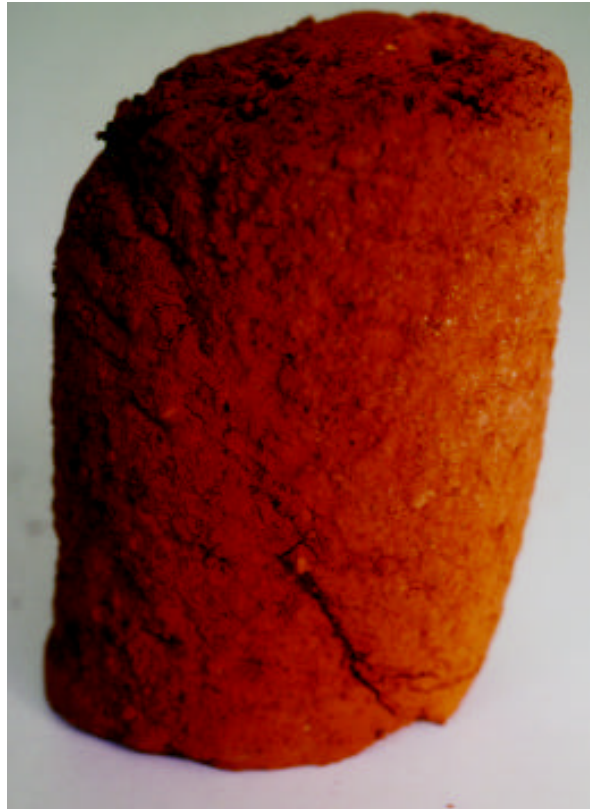
Figure 4.58: Undisturbed specimen after undrained triaxial test with an effective confining stress of 4500 kPa.
