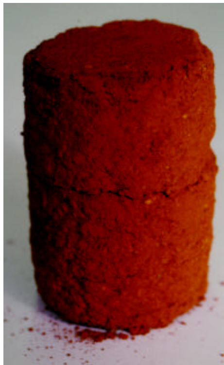
Figure 4.59: Undisturbed specimen after drained triaxial test with an effective confining stress of 3500 kPa.
