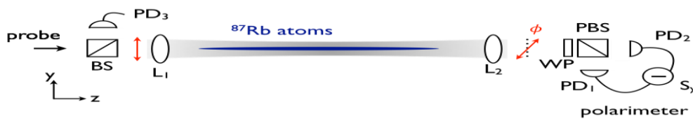
Figure 1: Schematic of the Atomic magnetometer set-up [6].
