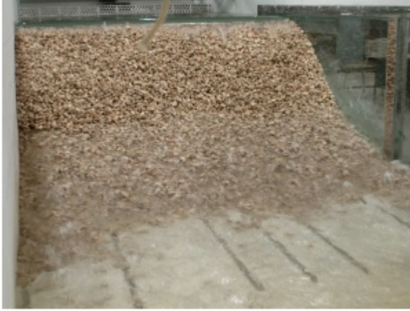
(a) Mass sliding failure
