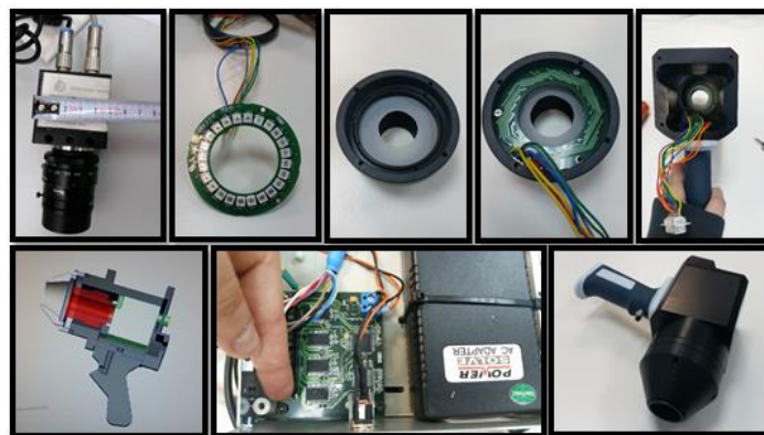
Figure 2. Camera, light ring, PVC case, mechanical design, power supplies and handled IR MS system.
