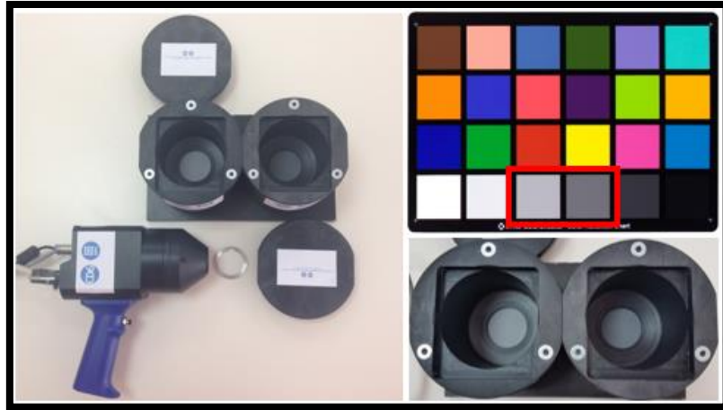
Figure 4. IR MS system base and color checker. The references chosen are highlighted in red.
