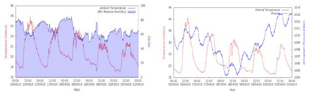
Figure 3 Data plot of a system test during a period of one week. On the left humidity with its own temperature sensor, on the right atmospheric pressure with its own temperature sensor
