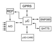
Figure 1. Schematic of the datalogger
