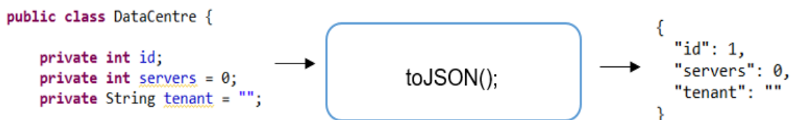
Fig. 15 Simple example of toJSON() method of GSON library
