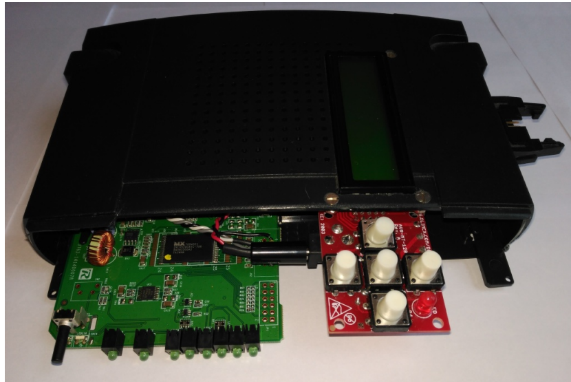
Figure 6.7: Detail of power input wired solidary to the router DC input (red and black braided wires)
