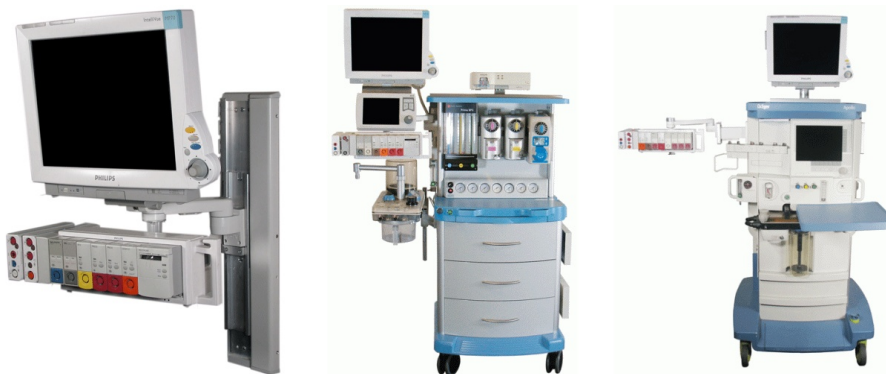
Figure 5.9: Different uses for MP70 monitor: bedside, anaesthesia and operation room configurations
