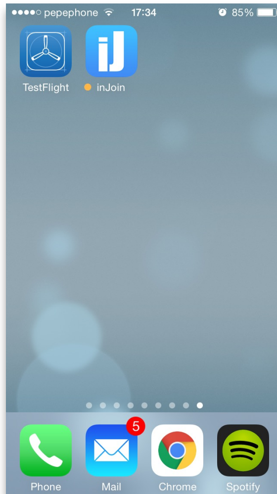
Figure 4.30: Successful Beta App installation via TestFlight (the orange dot identifies TestFlight-installed Apps) (iOS 8).
