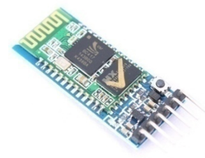
Figure 2.12 Typical TTL to Bluetooth module.
