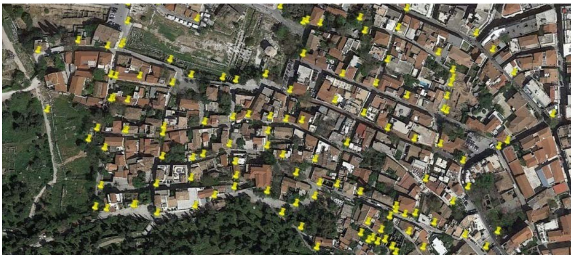
Figure 3.8 Ground Control Point (GCP) distribution.
