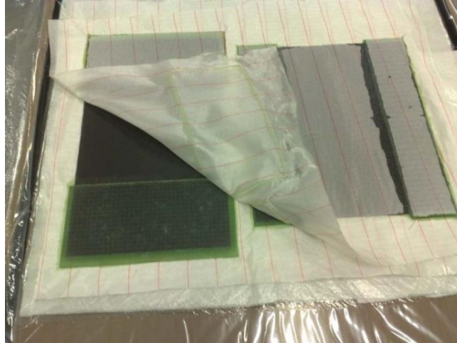
Figure A.8: PP-C/E-T-0 and PP-C/E-T-90 laminates with tabs after tab-adhesive curing (provided by NTNU).
