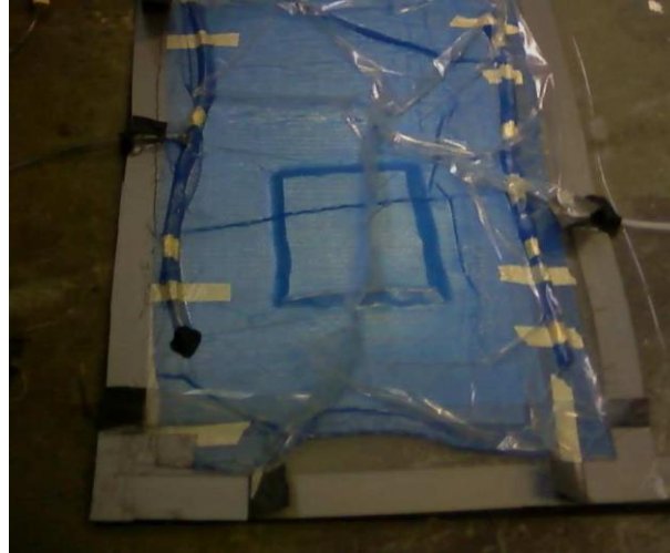
Figure A.1: Vacuum infusion of laminate (provided by AS2CON).
