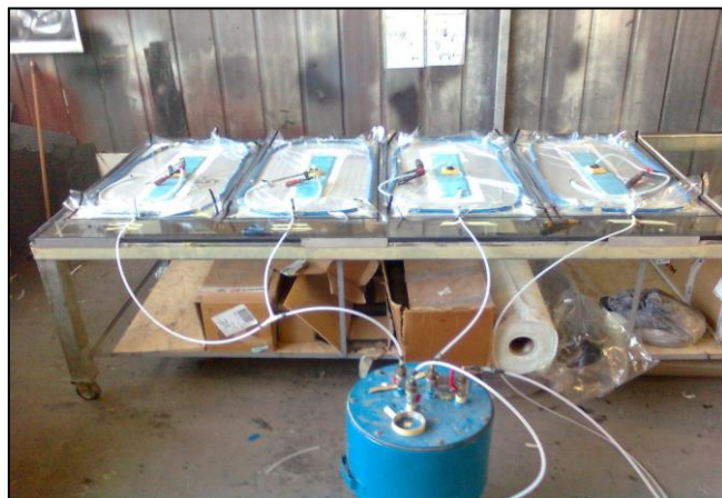
Figure 3.5: Manufacturing of P2D specimens' patches (figure provided by AS2CON).
