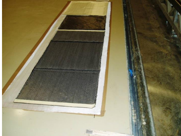
Figure A.3: Plies configuration prior to infusion (provided by UM).
