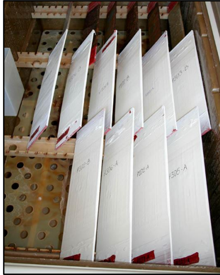
Figure 5.4: Painted P3 specimens placed into the environmental chamber.
