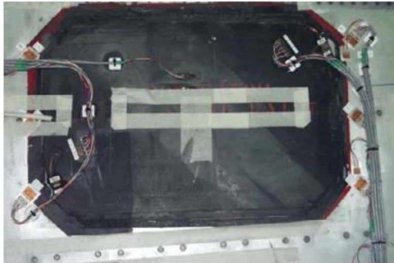
Figure 1.3: Patch with structural health monitoring system bonded to F-111 wing ( Baker et al, 2009 ).
