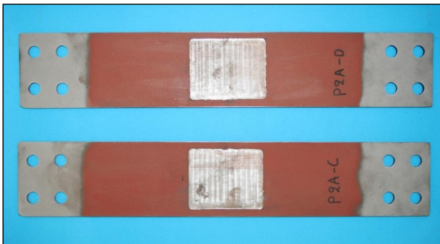
Figure 3.8: Thickness reduction of the central area of specimens P2A-C and D.
