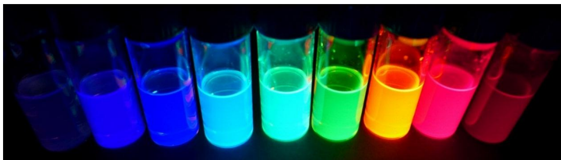
Figure 2-18: Cesium lead halide perovskite nanocrystals. Color change comes from changing the halide compositing: far left sample = \text{CsPbCl}_3 , Middle sample = \text{CsPbBr}_3 and far right sample = \text{CsPbI}_3 . Other colors come from different ratios of Cl:Br or Br:I.
