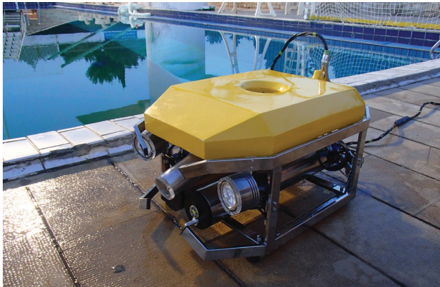
Figure 11. ROV during wet testing at the University swimming pool.
