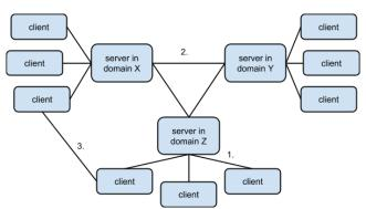
Fig. 5. Distributed client-server architecture of XMPP.
