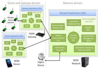
Fig.4. ETSI M2M functional architecture.
