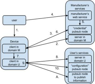
Fig 7. Example of using pubsub for device configuration.
