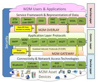
Fig. 2. Conceptual layers of technology relevant for M2M.
