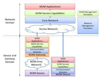
Fig. 3.ETSI M2M high level architecture
