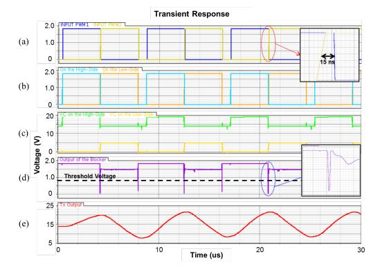
Fig. 8. Simulated voltage waveforms of the amplifier when 15 ns overlapping signals are connected to the output nodes of the dead-time generator: (a) Input overlapping signals, (b) inputs of the level shifters, (c) gate signals of the switching transistors, (d) output of the breakdown blocker, and (e) output of the amplifier. Block-box insets: Detail view of the input overlapping signals and the output of the blocker.
