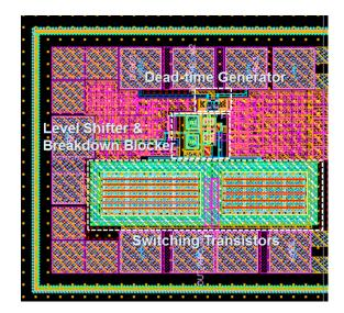
Fig. 3. Layout of the power amplifier with the proposed gate driver IC using TowerJazz's  $0.18 \mu m$  BCD process.
