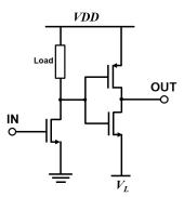
Fig. 4. Schematic diagram of the level shifter. The VDD is 5 V for the low-side switching transistor and AVDD for the high-side transistor. The VL is 0 V for the low-side and AVDD-5 V for the high-side.
