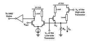
Fig. 5. Schematic diagrams of the breakdown blocker. The DVDD is the supply voltage of the digital logic circuits.
