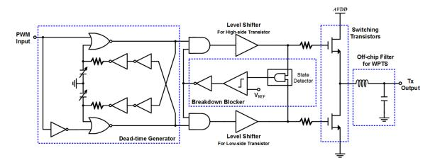
Fig. 2. Block diagram of the gate driver integrated circuit and the half-bridge power amplifier for the tightly-coupled wireless power transfer system (WPTS).
