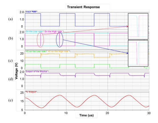
Fig. 6. Simulated voltage waveforms of the amplifier in Fig. 1 under normal conditions: (a) Input PWM signal, (b) outputs of the dead-time generator, (c) gate signals of the switching transistors, (d) Output of the breakdown blocker, and (e) output of the amplifier. Block-box insets: Detailed view of the outputs of the generator.
