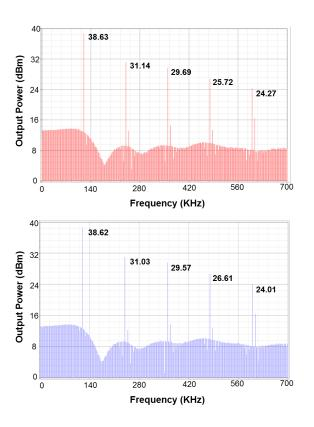
*Fig. 11. Output power spectrum of the power amplifier:* (*upper*) without the operation of the breakdown blocker and (lower) with the operation of the blocker.
