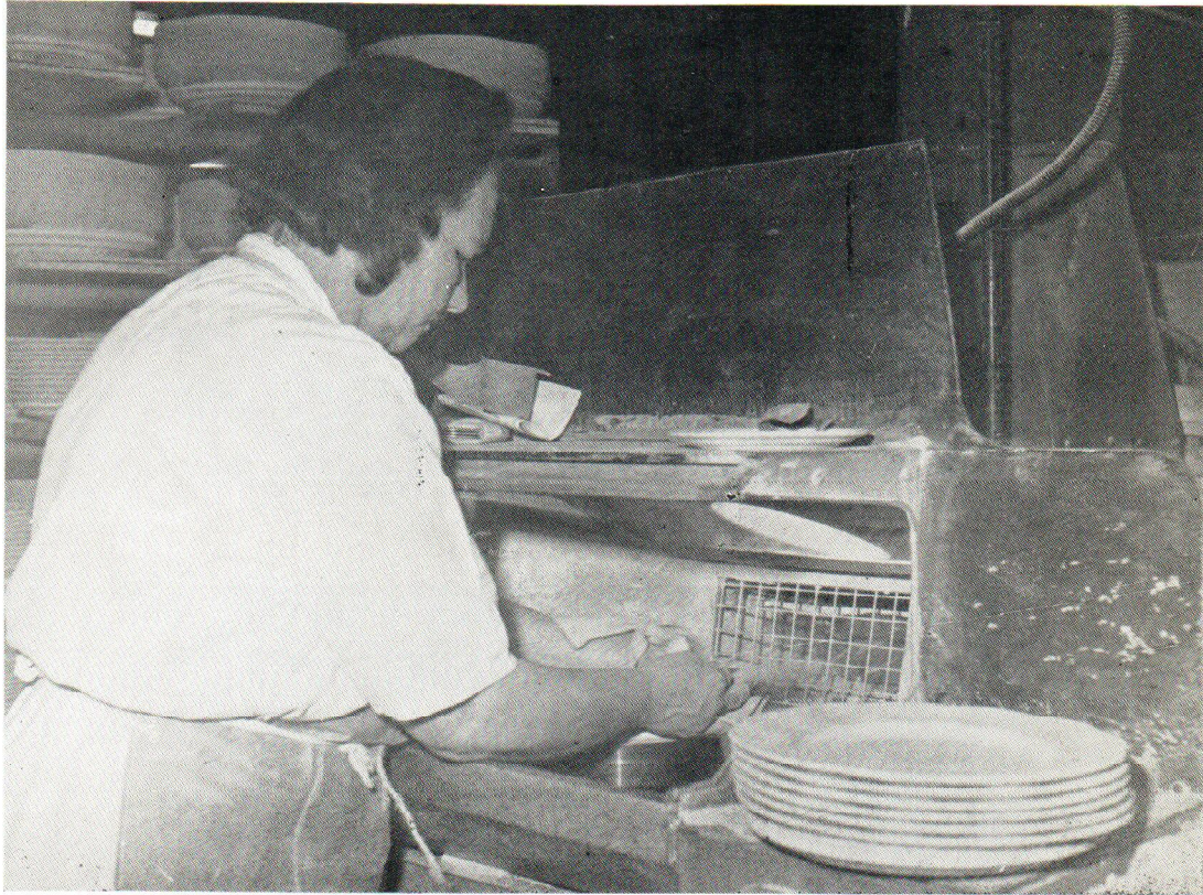
Fig. 2. Fettler working with improved towing hood designed by British Ceramic Research Association.
