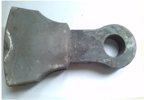
Figure 5. The hammer casted by optimized process.
