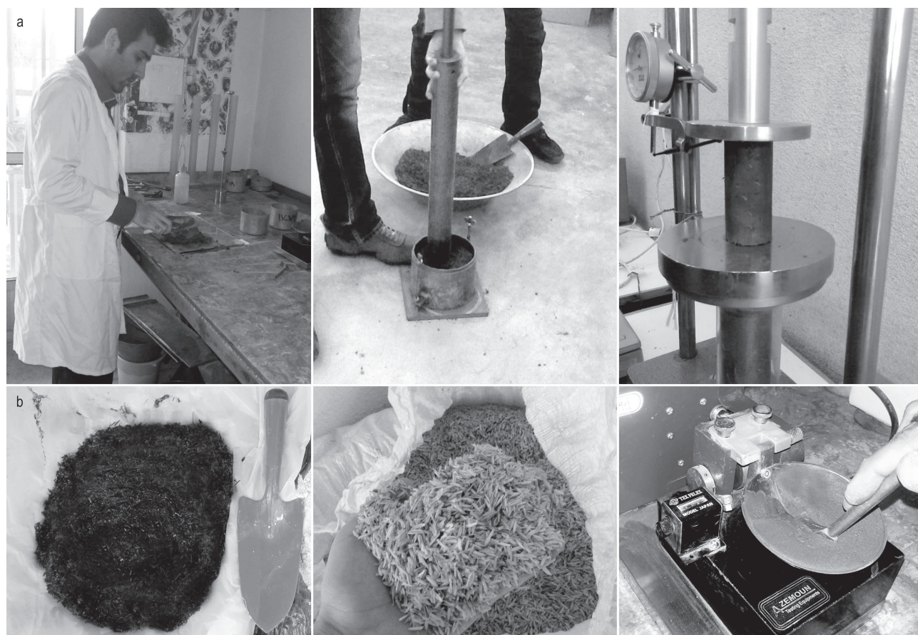
Fig. 2 Laboratory tests to identify specification of different combinations (a) and produced RHA and rice husk (b)
