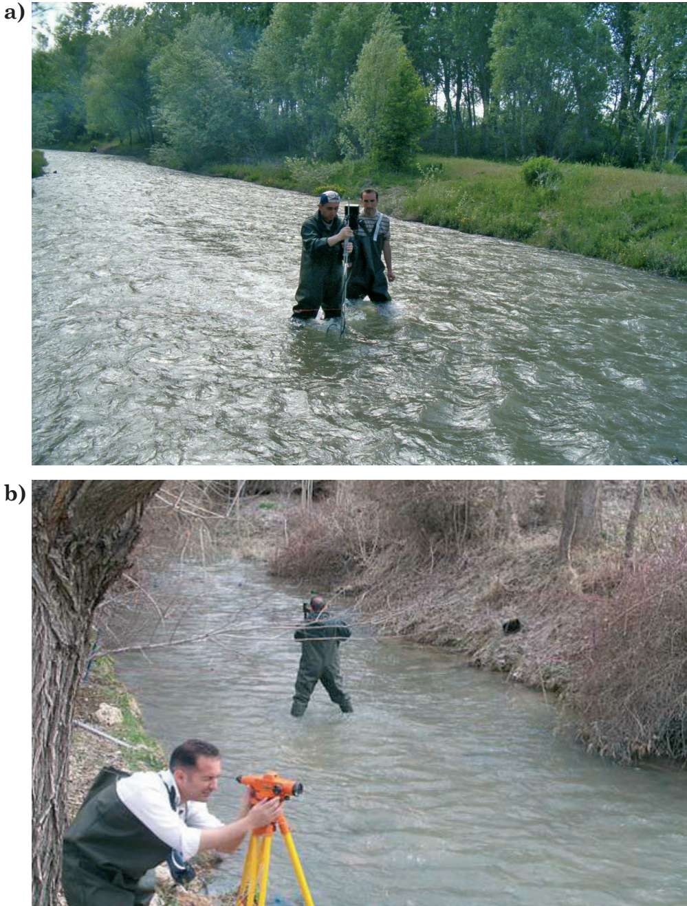
Figure 2. Velocity and topographical measurements at (a) Barsama and (b) Şahsenem Stations (Ardiclioglu et al. 2012).
