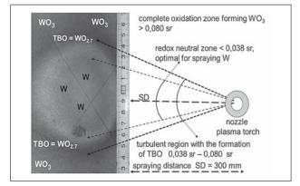
Figure 4 Evaluation scheme of footprint deposition tungsten by thermal spraying
