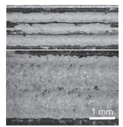
Figure 11 (a) Gradual coating of W-wires d = 0,8 mm with corundum ceramics, poor adhesion in the original, (b) improve adhesion to the WSi, surface
