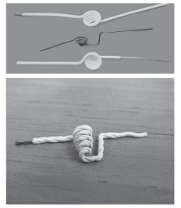
Figure 12 Example of practical application protective heating of W-coils for steam apparatus
