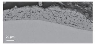
Figure 3 Cross-section of tungsten wire with WSi<sub>2</sub> coating
