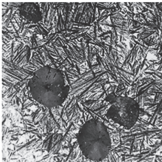
Figure 1 Microstructure of the cast iron (ADI), magn. 400x
