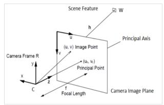
Fig. 10: Pinhole camera model
