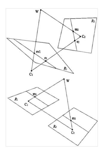
Fig. 11: Epipolar rectification
