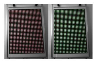
Fig. 5: Centers of markers on left and right camera images
