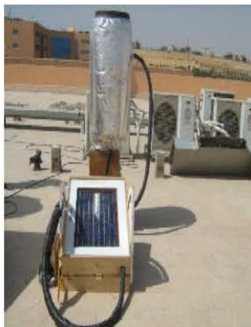
Fig. 2 Thermosyphon effect used on PV/T system, [15]
