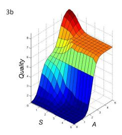
Figure 3. Effect of the print parameters on its quality: image positioning (L) and color difference (E) (a), reproduction of a raster dot (S) and adhesion of ink layer (A) (b).
