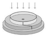
Figure 1. Test specimen in ring formation of RCT method
