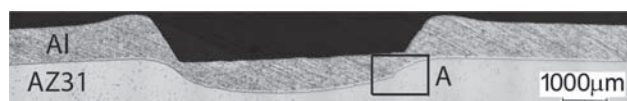
Figure 5 A two-layered AZ31 - Al sample after the compression test at a temperature of 300 °C and strain rate of 0,1 s -1 .
