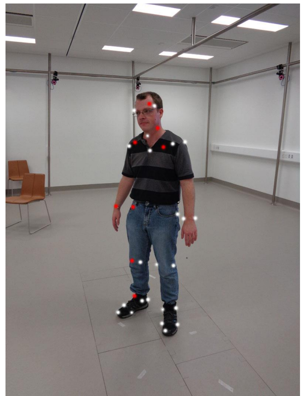
Figure 3. Body with markers suitable for Maya pivot rigging (white markers are directly visible, red markers are included to indicate the corresponding marker that is masked or out of view). Note 3 of 10 Vicon Bonita cameras are visible in the background.
