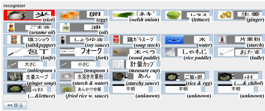
Figure 7: Interface for wizards. When a button for object o is pushed, a(o) = \text{'touched'} is sent with a timestamp. Then, the button turns red. a(o) = \text{'released'} is sent after pushing the red button again.
