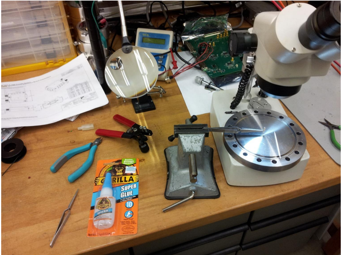
Figure 8.12. Typical setup for gluing etched tips to tuning forks.
