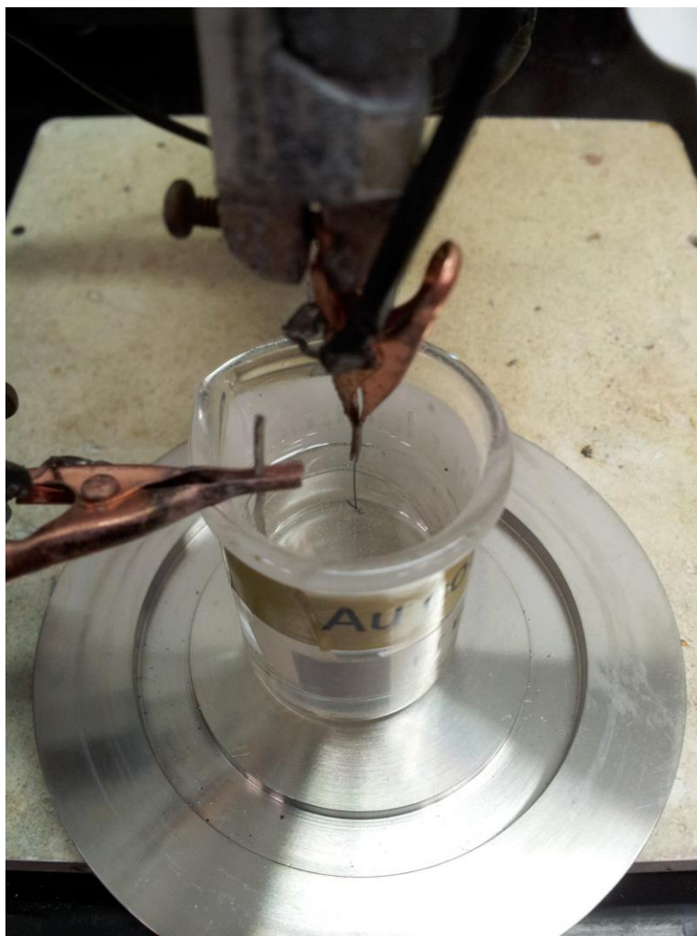
Figure 8.11. Close-up of the W etching in 8 M KOH.
