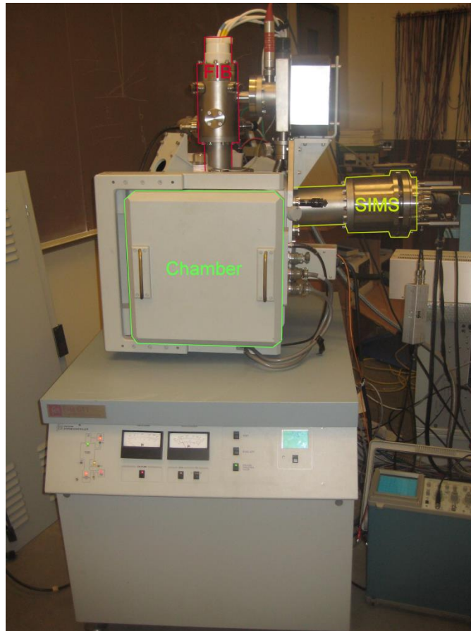
Figure 7.1. FIB 611 vacuum console showing air isolation table, chamber, 2LI FIB column and SIMS-I analyzer.
