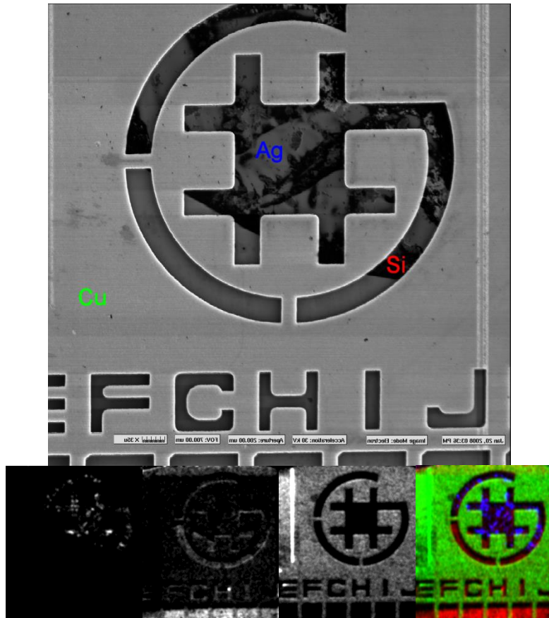
Figure 3.3. Sample of a three-species SIMS composite image. The contributing images have been registered, Gaussian blurred and histogram stretched in order to create the final colored image. (bottom row images, left to right) Au, Si, Cu and composite.
