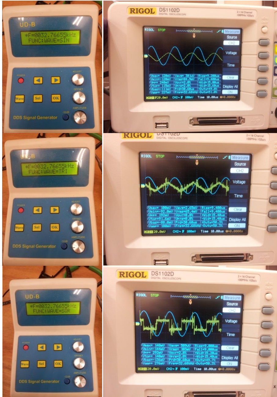
Figure 4.5. Illustration of the resonance phenomenon for a quartz tuning fork in its sealed can using a function generator. The yellow curves are the excitation and the blue are the tuning fork response which is always sinusoidal. (top) Sinusoidal excitation. (Middle) Triangle wave excitation. (Bottom) Square wave excitation.
