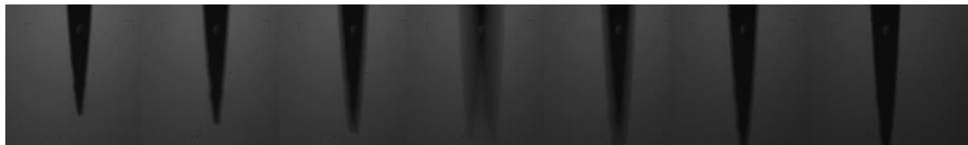
Figure 5.7. Direct measurement of an AFM tip mounted on a tuning fork. The tuning fork was driven using 200 mV P-P. Normal operation is typically 2-7 mV r.m.s. Image horizontal field of view is approximately 7.5 \mu\text{m} . This is sample #19. 1740 images were extracted from the acquired video for analysis. The large difference between Q measured electrically and from video are still not understood entirely. This experiment demonstrates the feasibility of using ETEM only qualitatively so far.
