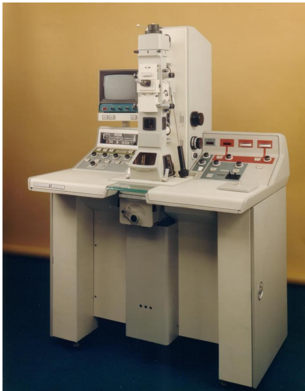
Figure 5.3. (left) Photograph of the electrostatic transmission electron microscope used in this work. (right) Drawing of the ETEM optics. This system was designed by Gert Rempfer in the 1970's for applications in biology. It has some features which were innovative for the time, including 3D visualization using shutter glasses. (images reproduced from original product brochure)
