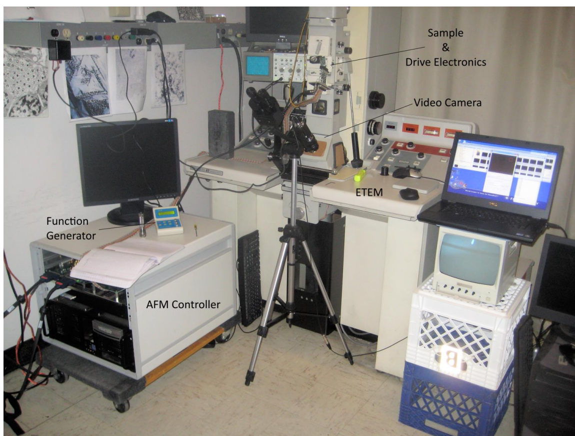
Figure 5.5. Setup for recording video of vibrating AFM tips inside the ETEM. Initially, the AFM controller was used to drive the tuning fork. Later the UD-B Direct Digital Synthesis (DDS) function generator was used.
