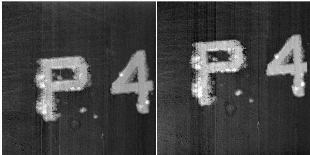
Figure 9.10. (left and right, respectively) Trace and retrace images (50x50 \mu\text{m}^2 ) of one of the first unambiguous scans on a MetroCal wafer in air (shown in Figure 9.9). The fast scan axis is shown along Y. Some processing was performed to align the scan lines and to level the vertical scale. Some distortion is evident along the fast scan axis. This is a result of operating the XY scan bed in open-loop mode.
