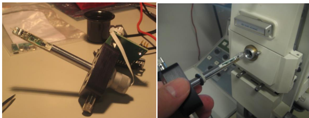
Figure 5.4. Photograph (left) of the ETEM sample holder which has been modified to hold tuning fork based AFM sensors, including the MESFET and scan head preamp. Photograph (right) showing a tuning fork being inserted into the ETEM.
