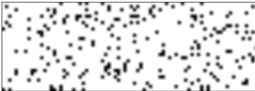
Figure 3.14: Random \mathbf{Y} matrix with black dots indicating the spatiotemporal code for when a crossbar can integrate an input signal.
