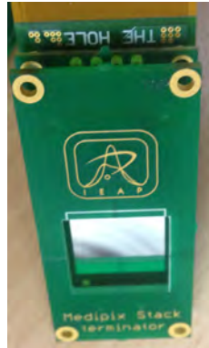
Figure 7.11: Close-up view of the Medipix detector protection.
