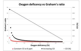
Figure 3: Oxygen Deficiency against Graham's ratio at a constant CO value (8 ppm) and variable CO
