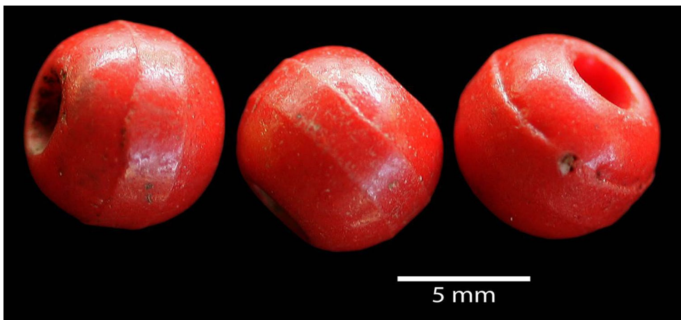
Fig. 1 Three beads coloured with nano- (Zn, Cd) S_xSe_{x-1} mixed crystals
